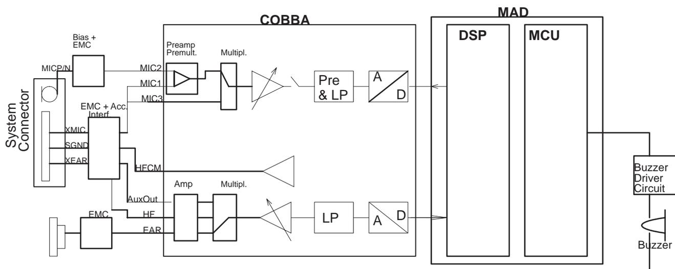
The baseband supports three microphone inputs and two earphone outputs. The inputs can be taken from an internal microphone, a headset microphone or from an external microphone signal source. The microphone signals from different sources are connected to separate inputs at the COBBA-GJ asic. Inputs for the microphone signals are differential type.
