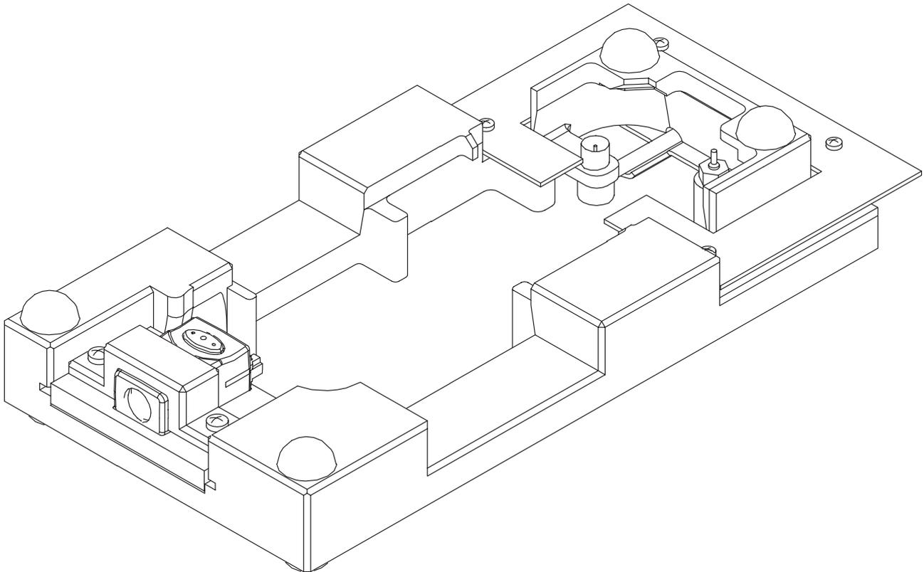
\*) Connect the External antenna cable XRC-1B, service Cable SCH-5, and the DC Cable PCS-1 to the JBT-1 jig.
