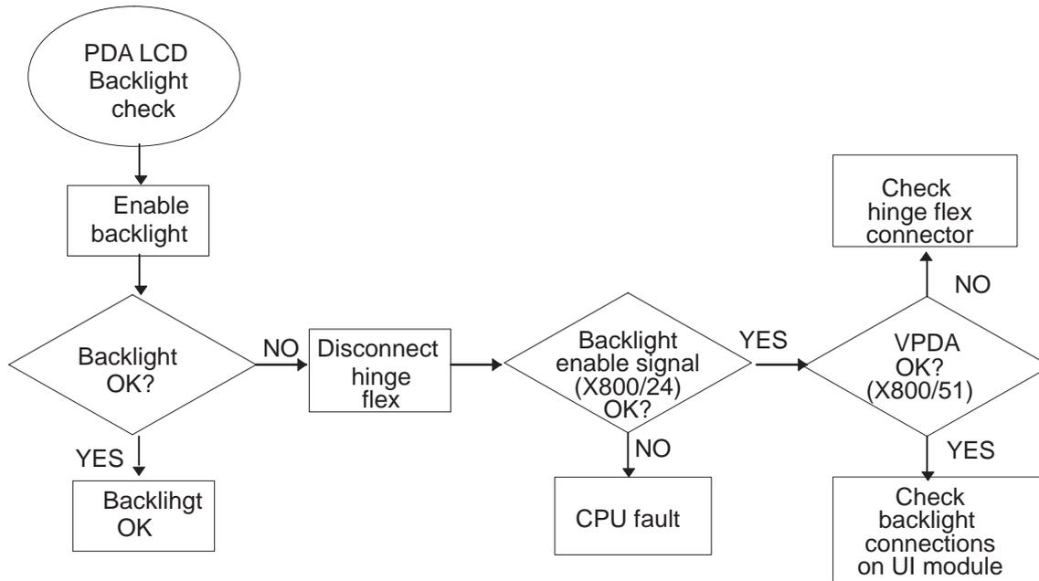
Figure 27. PDA LCD backlight troubleshooting
