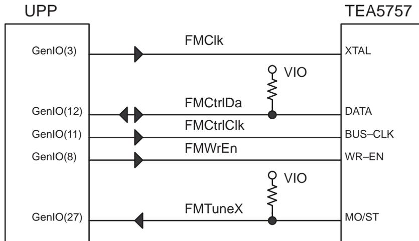
NOTE: *FMCtrlClk* needs to be set to logic '1' when data is not written or read. This is required for correct operation of the *FMTuneX* signal.
