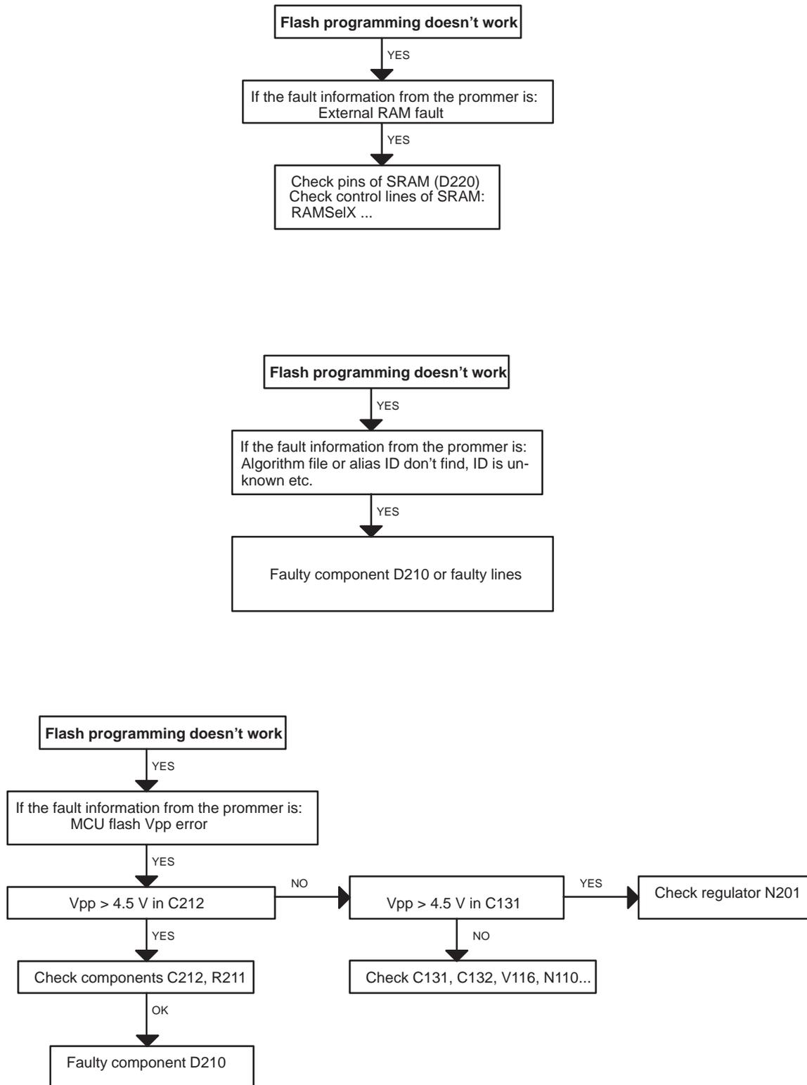
Figure 11. Troubleshooting Diagram for Flash programming doesn't work (via system connector X170)
