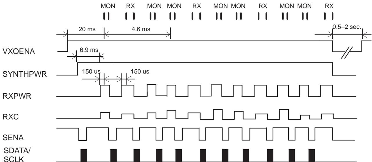
Synthesizer Timing / IDLE 2, frame can start from RX-burst
