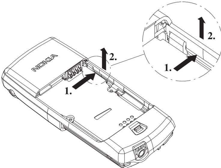
Step 1. Push c-cover edge outwards to release it behind locking snap
