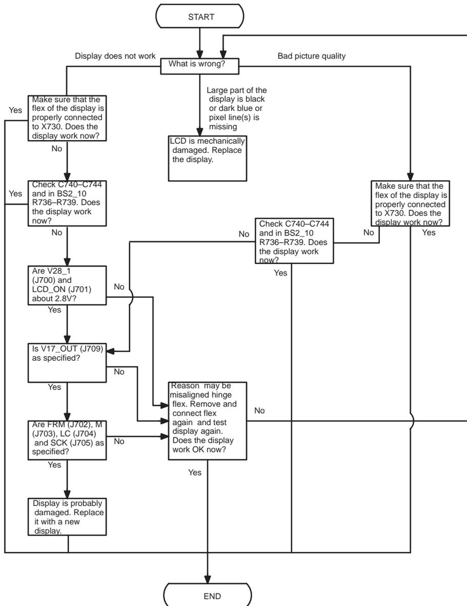
Figure 40. Flowchart for troubleshooting of the PDA LCD.
