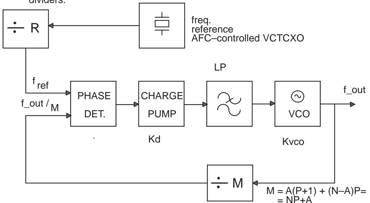
LO-signal is generated by SHF VCO module. VCO has double frequency in DCS1800 and x 4 frequency in EGSM compared to actual RF channel frequency. LO signal is divided by two or four in HAGAR (depending on system mode).
