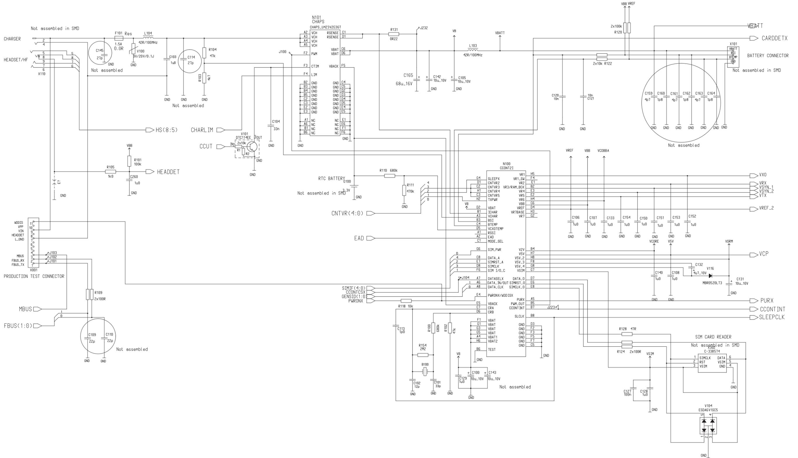
**Circuit Diagram of CPU Block** (Version 12.03 Edit 14) for layout version 12
