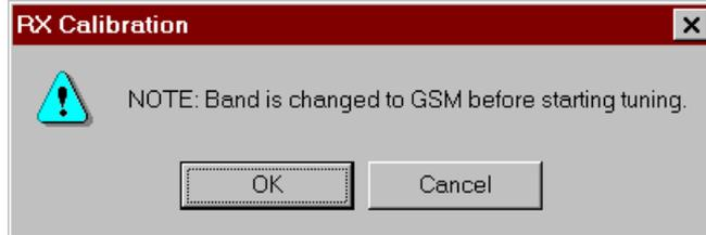
Tuning is automatically continued in GSM 1900 band, after saving tuning values in GSM 900 band. If tuning was started in GSM 900 band, user is asked to continue tuning in GSM 1900 band.
