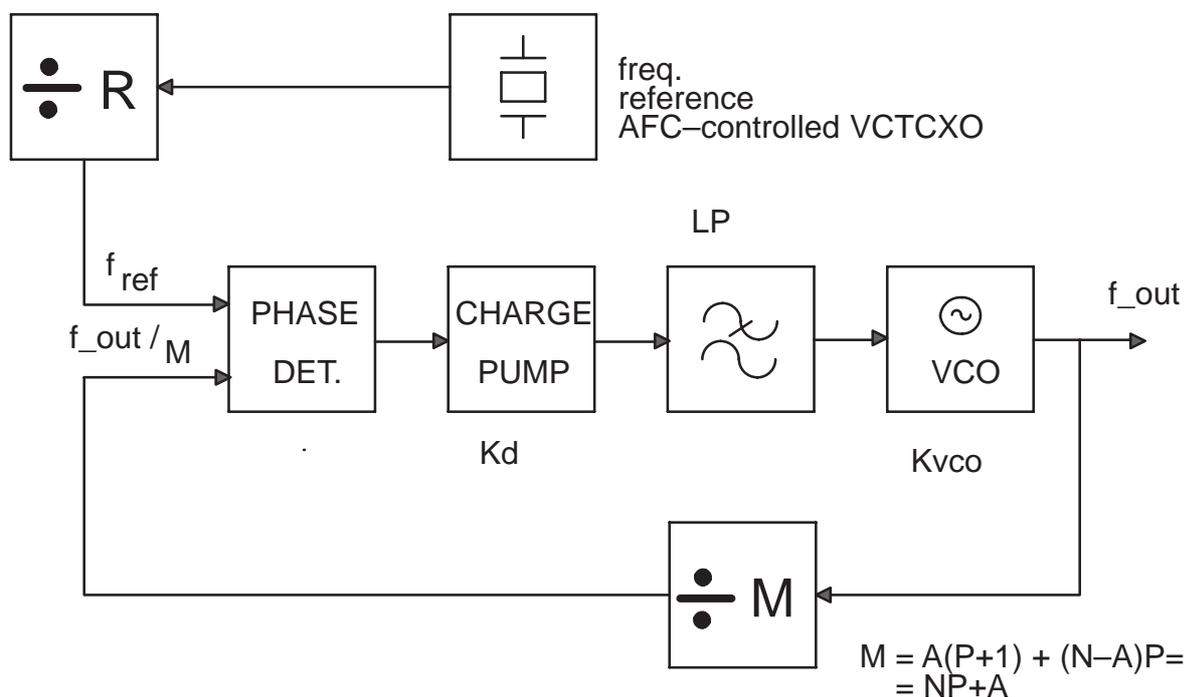
VHF PLL is also located into PLUSSA. There is 16/17 ( P/P+1 ) dual modulus prescaler, N- and A-dividers, reference divider, phase detector and charge pump for the loop filter. VHF local signal is generated with a discrete VCO-circuit. VHF PLL works in the same way as UHF-PLL. VHF-PLL is locked on fixed frequency, so higher reference frequency is used to decrease phase noise.
