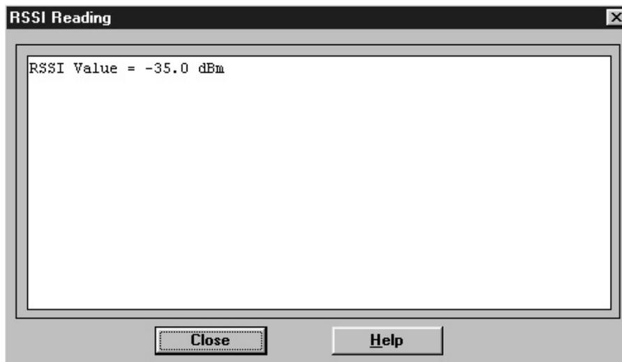
RSSI value is read continuously until user presses ESC-key or Close button to cancel reading.
