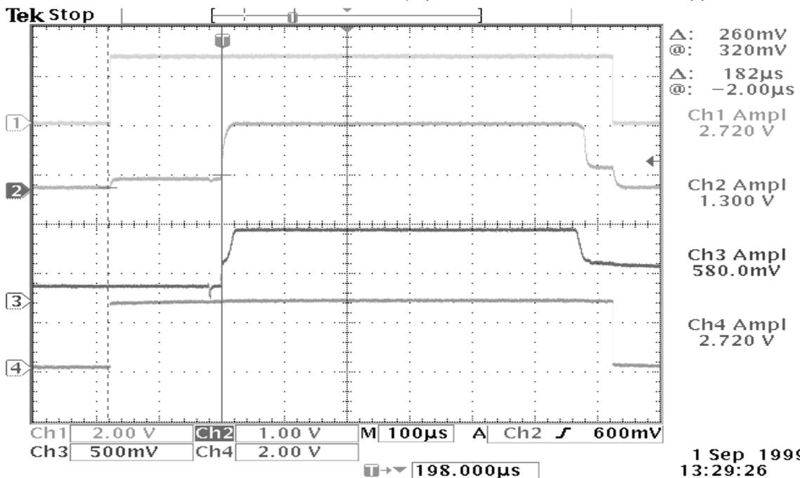
**Picture 5. VBATT during TX burst**
