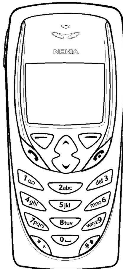
The NHM-7 is a dual band transceiver unit designed for the GSM900 (including EGSM) and GSM1800 networks. It is both GSM900 phase 2 power class 4 transceiver (2W) and GSM1800 power class 1 (1W) transceiver.
