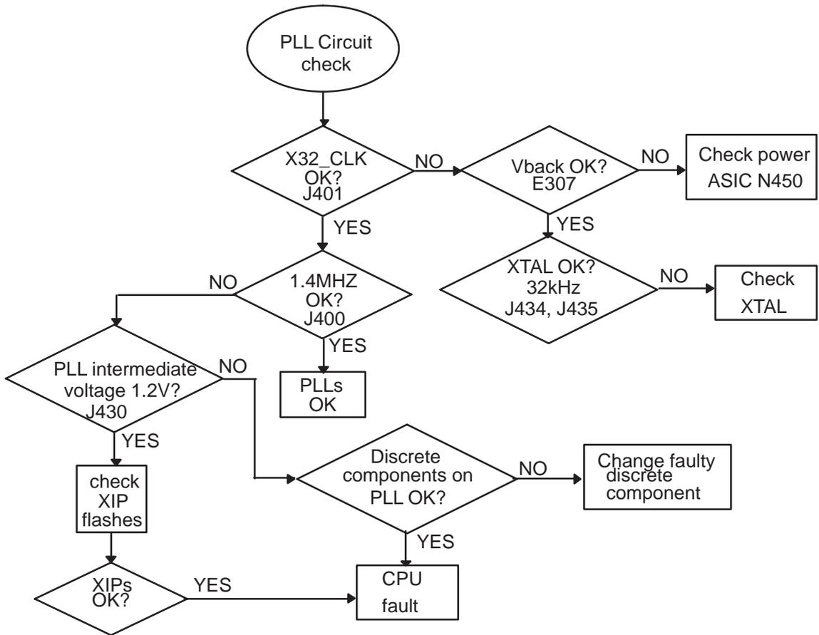
Figure 23. PLL clock generation circuit check
