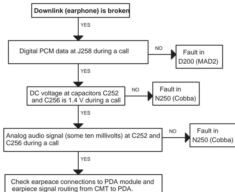
Figure 7. Trouble Shooting Diagram for Audio Failure
