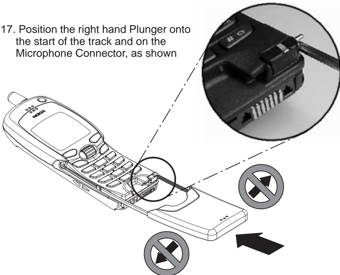
18. Position the left hand Plungers onto the start of the track and push the Slide Assembly into the phone.
