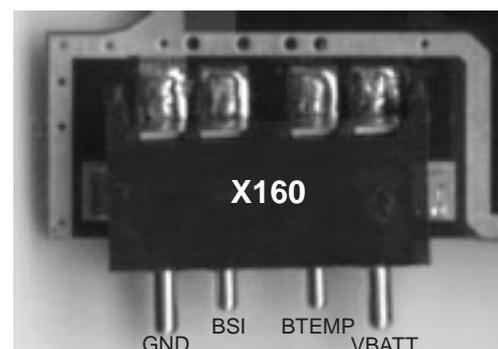
Figure 5. Battery Connector
