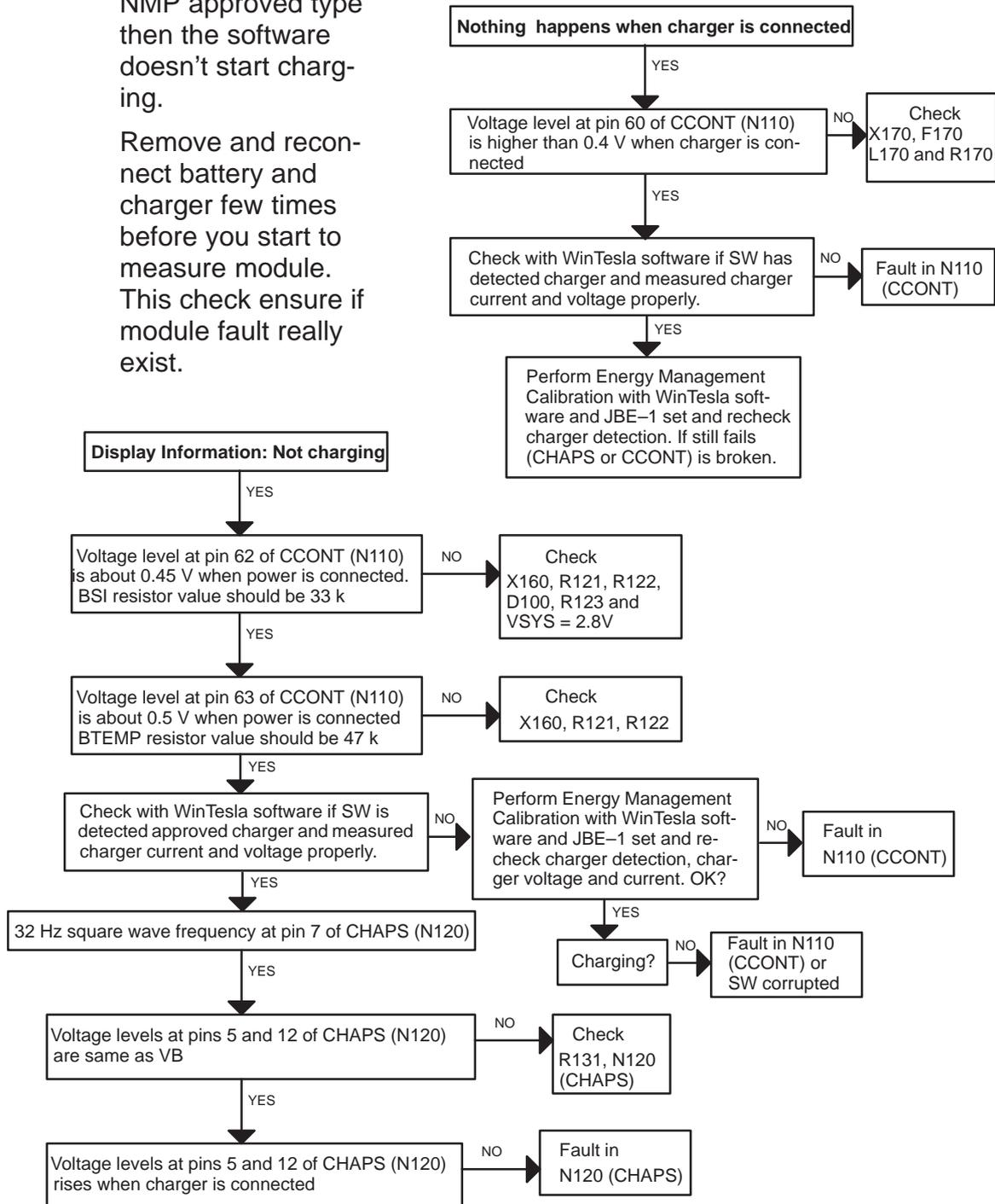
Figure 8. Trouble Shooting Diagram for Charging Failure
