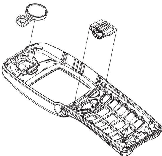
15. Remove the Speaker and the Roller Key
