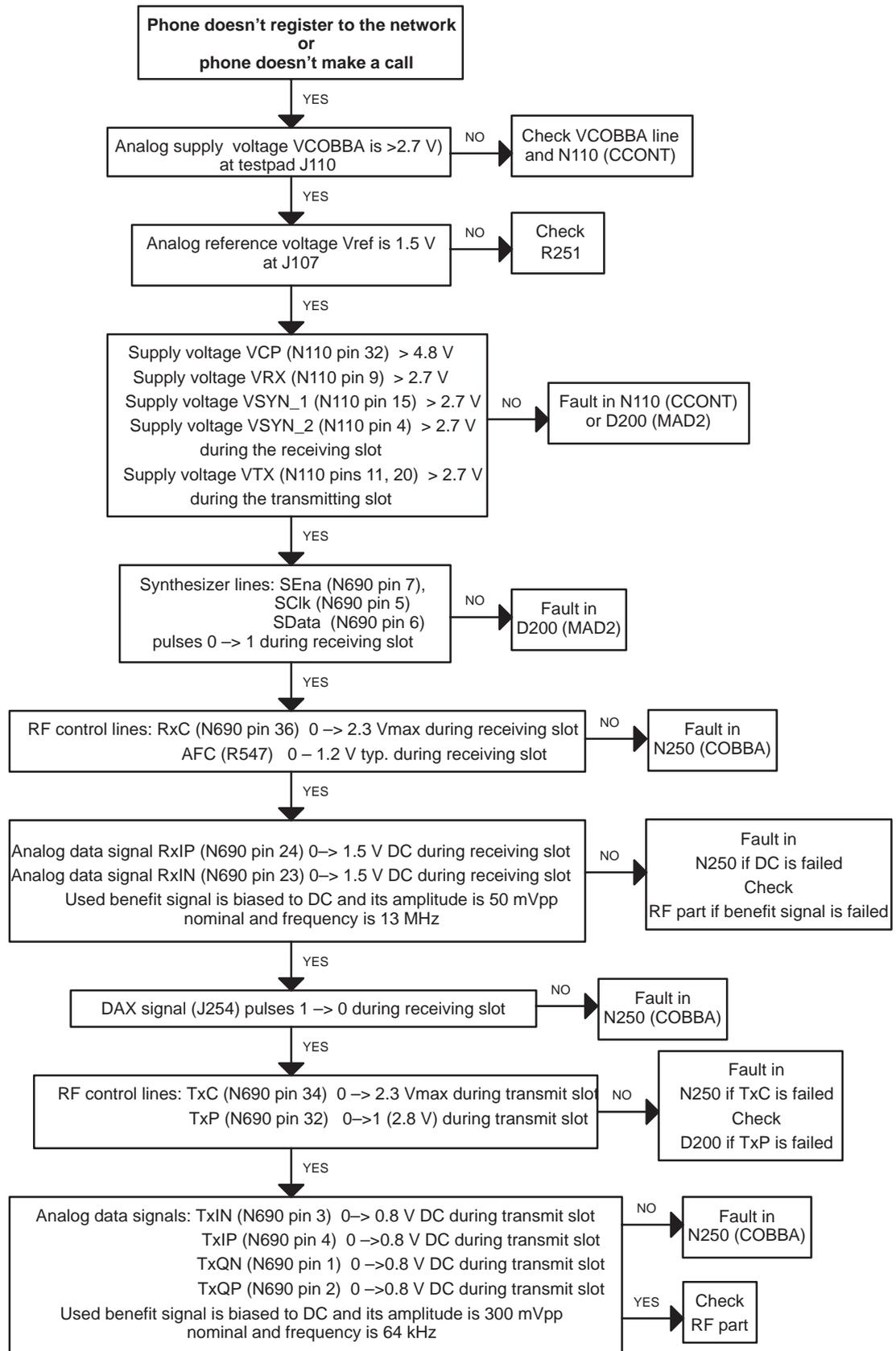
Figure 4. The phone doesn't register or doesn't make a call
