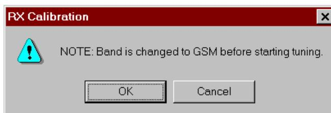
If PCN band was selected, when tuning was selected, tuning is automatically continued in PCN band, after saving tuning values in GSM band. If tuning was started in GSM band, user is asked to continue tuning in PCN band.
