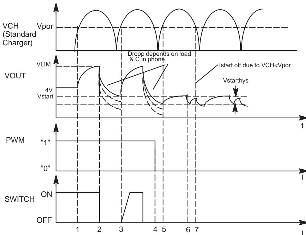
1. Battery removed, (standard) charger connected, VOUT rises (follows charger voltage)
