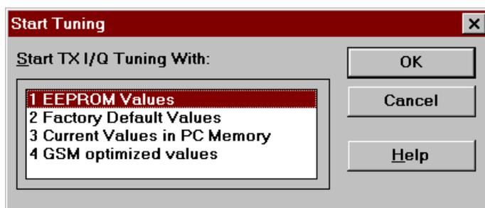
If user selects **4 GSM optimised values**, then tuning is started with values that were saved earlier in GSM band. Note that this selection is available only in PCN mode and when GSM values have been saved to PC memory.
