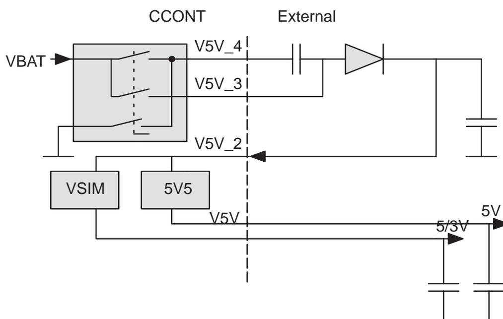
Figure 16. Principle of the SMR power functions
