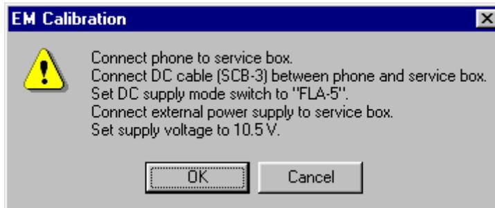
When power is connected and user selects Yes to continue, the application displays the **Energy Management Calibration** dialog box:
