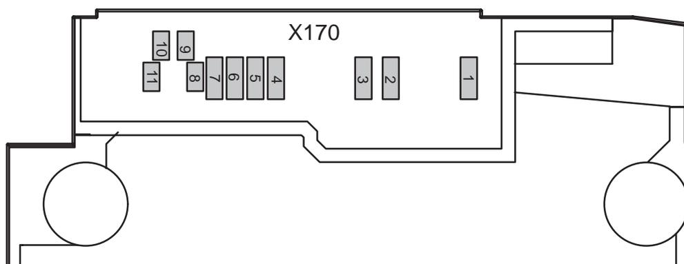
Figure 3. Bottom connector pads in BS8 module
