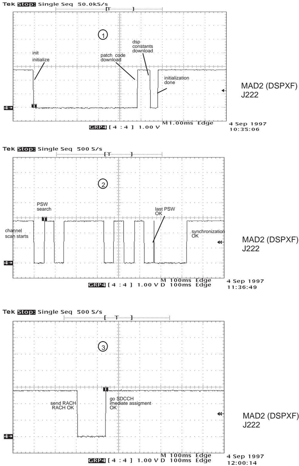
Figure 3. The states of DSP after power on
