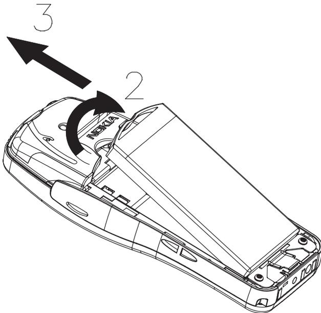
Rotate around the end of the battery and remove it upwards according to 3.
