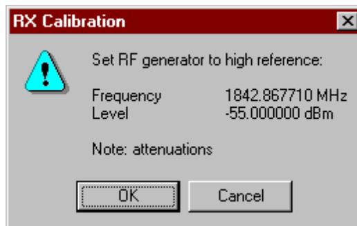
When the user acknowledges by pressing OK, the calibration with high input level is executed.
