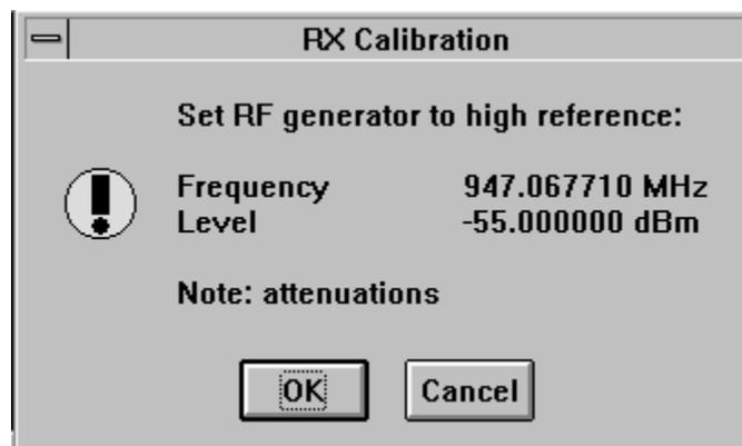
2. Measurement with high input level is executed
