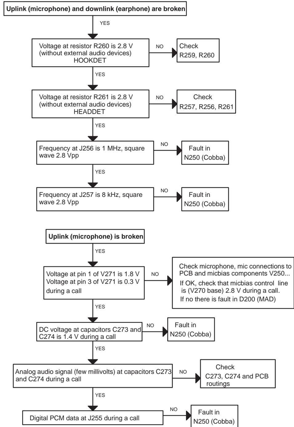
Figure 6. Trouble Shooting Diagram for Audio Failure
