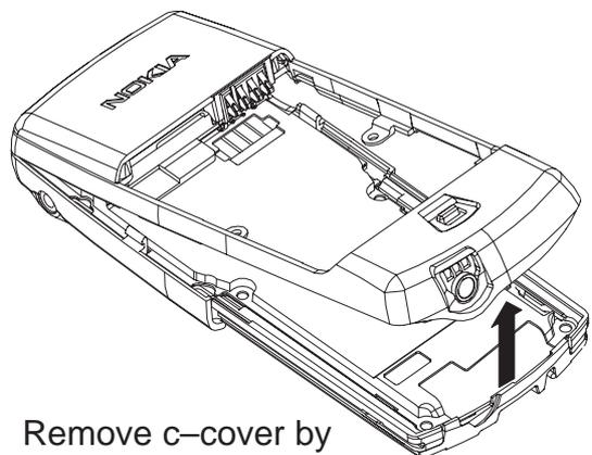
Remove c-cover by lifting up rear and pulling cover out.
