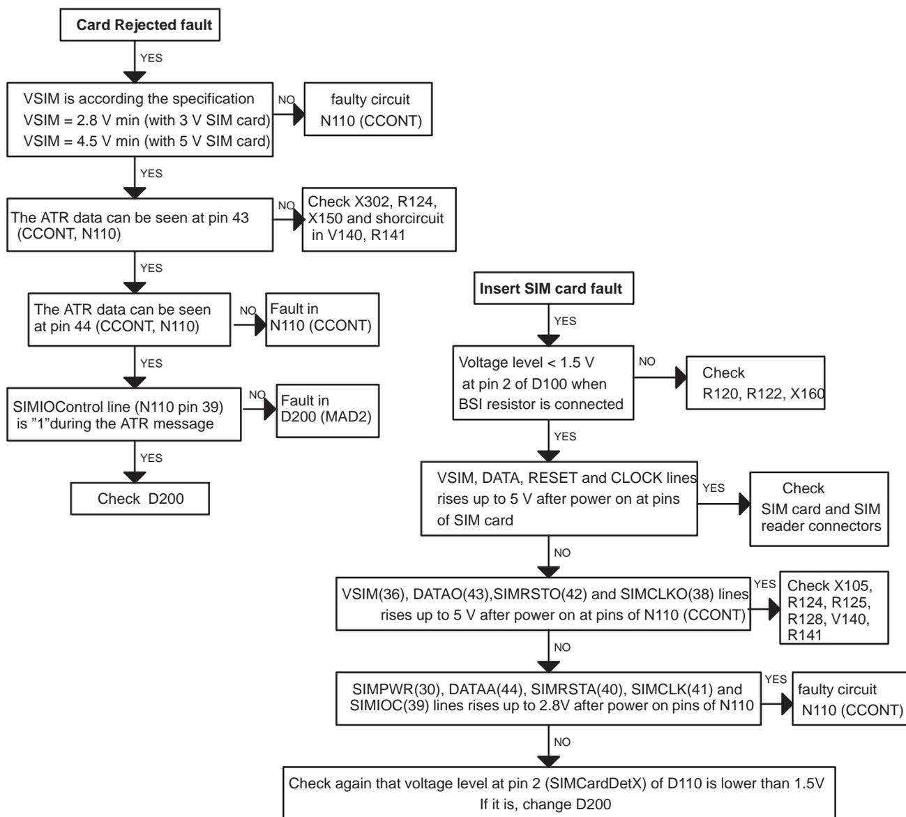
Figure 5. Troubleshooting for SIM card faults
