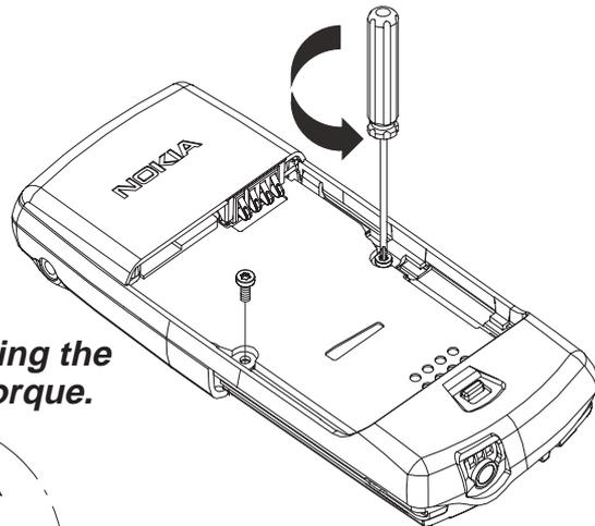
**NOTE: When assembling the screws, use 17 Ncm torque.**
