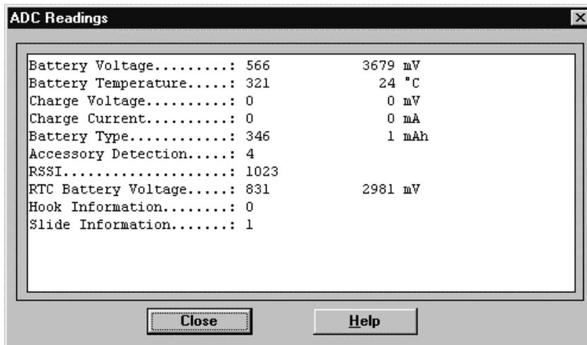
ADC Readings dialog has static text field where measurements are updated to window every one second.
