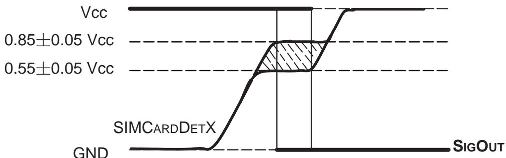
Figure 11. SIMCardDetX detection levels
