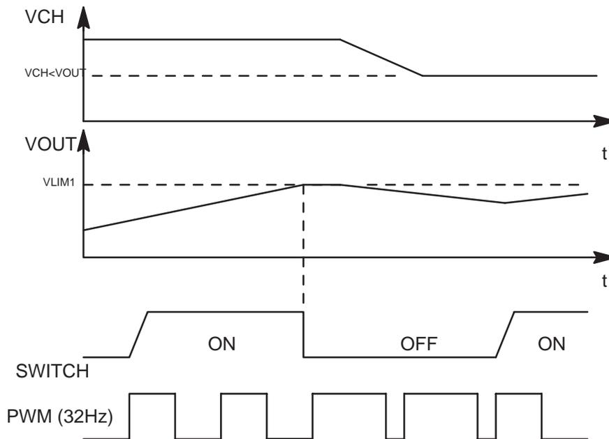
Figure 13. Output overvoltage protection( in principle; not in timescale)
