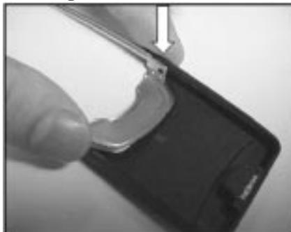
Push the Metal Slide onto the snap on one side of the Slide Cover.
