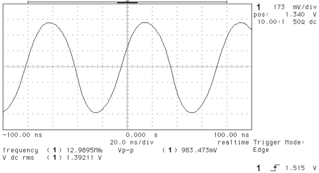
Picture 1. 13 MHz Main clock – signal
