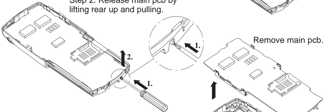
Step 1. Lift slide frame from bottom and loosen it from a-cover.
