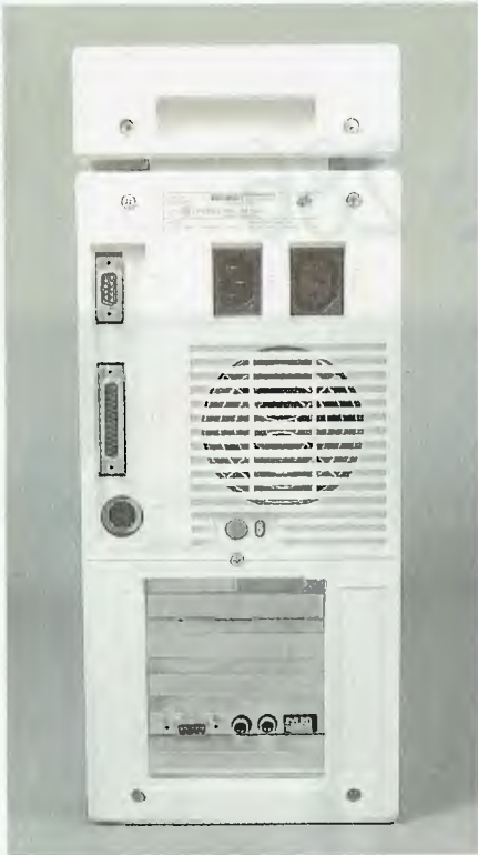
Figure 2. While the system comes standard with only one serial and one parallel port and only three unused slots (all 16-bit), expansion is provided for on the mother board.
