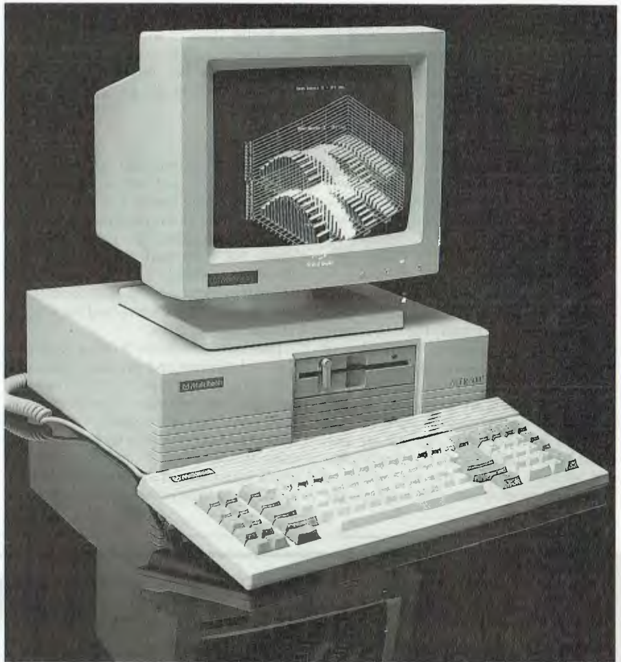
Figure 1. The Acer 500+ comes in three configurations. Standard with all three are one serial port, one parallel port, a games port and a clock/calendar. All include a paper white monitor compatible with the IBM mono display adapter and Hercules boards. The video board can be switched for Hercules monitors or CGA colour monitors.
