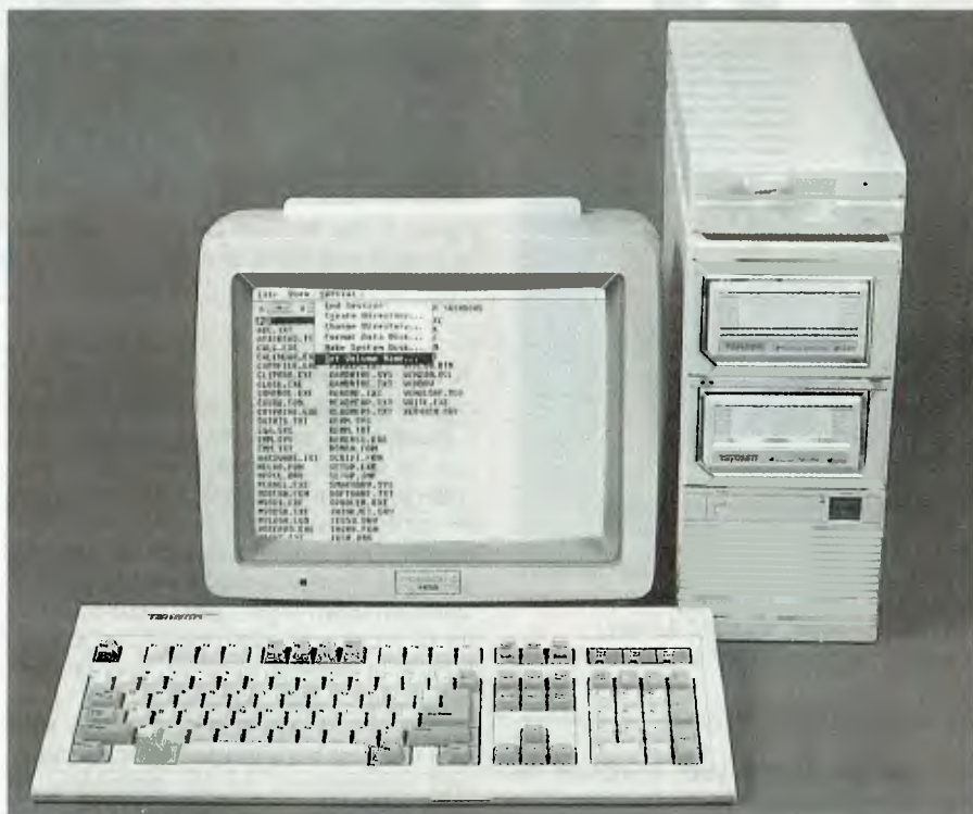
Figure 1. Tandon has packed a lot of innovation into the Pac 286. For example, its engineers have gone along way towards overcoming one of the major shortcomings of the 80286 with the memory mapper, which enables the machine to run constantly in real mode rather than protected mode.
