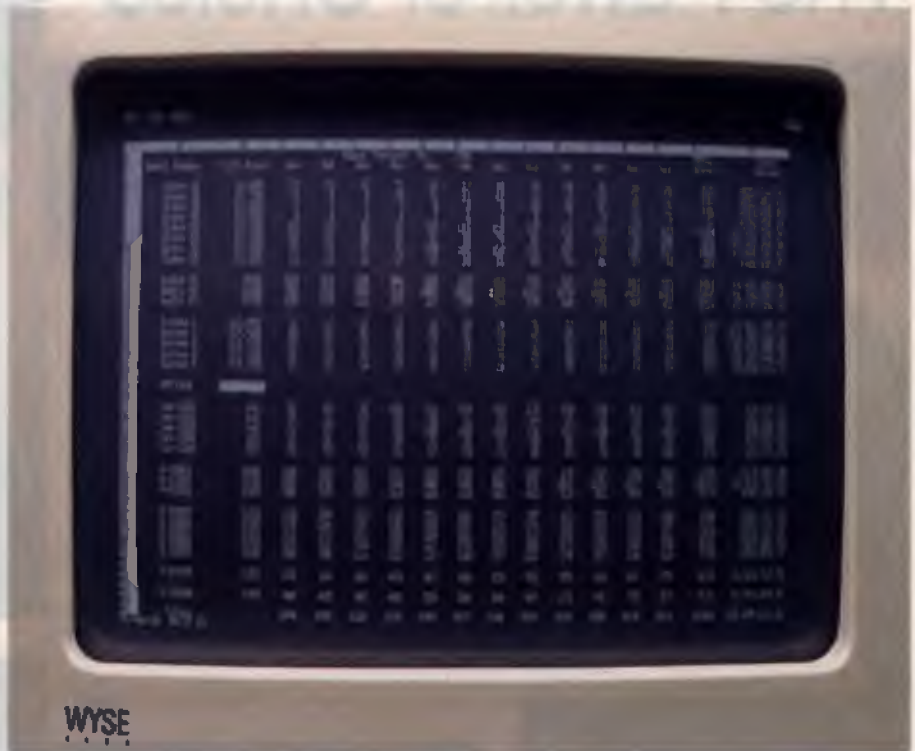
Figure 3. The Wy700 monitor has a 280 x 200 mm screen. It can be used as a high resolution (up to 1280 x 800 pixels) white monitor, as a CGA or as an IBM monochrome monitor.
