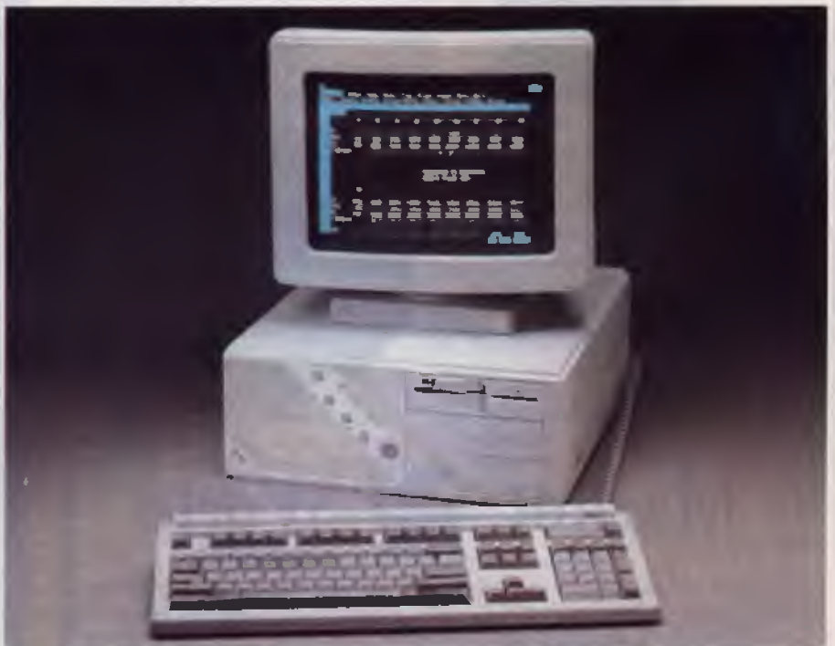
Figure 2. The Wyse 286 has a noticeably smaller footprint than the typical AT or the Wyse 386. The backlit LCD display is at a 45 degree angle and two more push buttons flank the date/time and CPU usage buttons – these are a reset switch, and a push button for power on/off.
