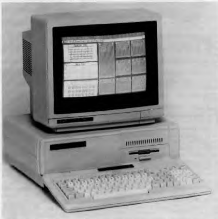
Figure 1. The 1000 TX from Tandy has an 80286 processor running at 8 MHz. Personal Deskmate 2 software is included in the basic price.
