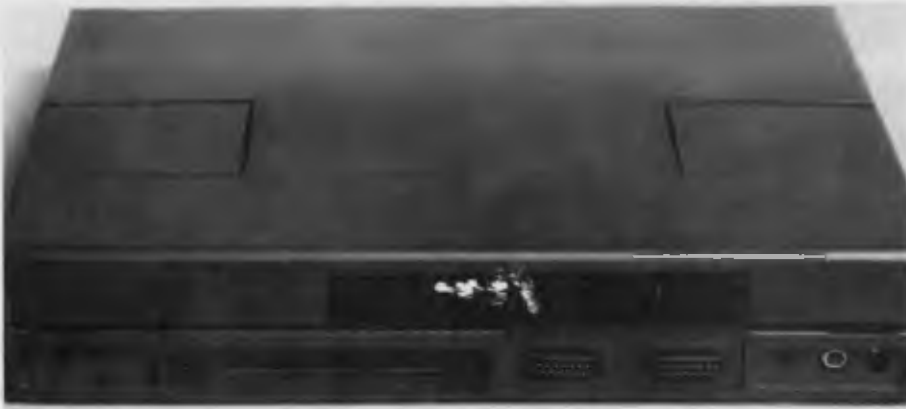
Figure 2. The Kookaburra offers one parallel and two serial ports plus an RS232 plug and connection for an external monitor.
