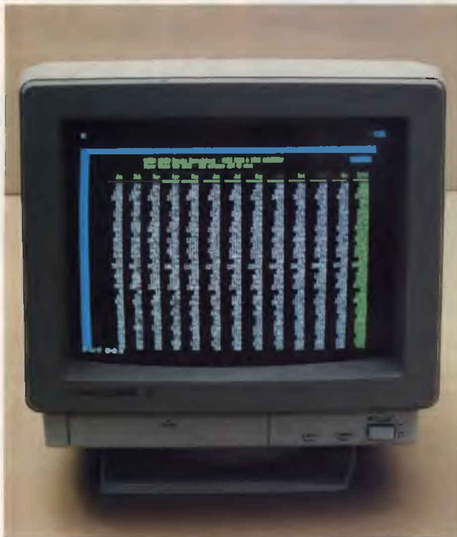
Figure 1. The Multisync II comes on a tilt and swivel base with the most used controls behind a flip down door on the panel under the screen. Note Lotus 1-2-3 with 132 columns and 44 rows.
