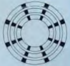
Figure 1* Perfectly aligned tracks. The black areas are "read only." These store critical track and sector ID information. The white areas are data sectors and store your system, programs and data.
