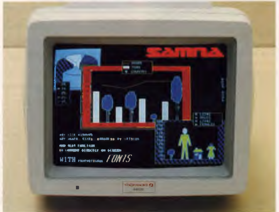
Figure 3. In EGA mode, the Thompson 4470D monitor offers the same resolution as the Multisync, as well as four text colours.
