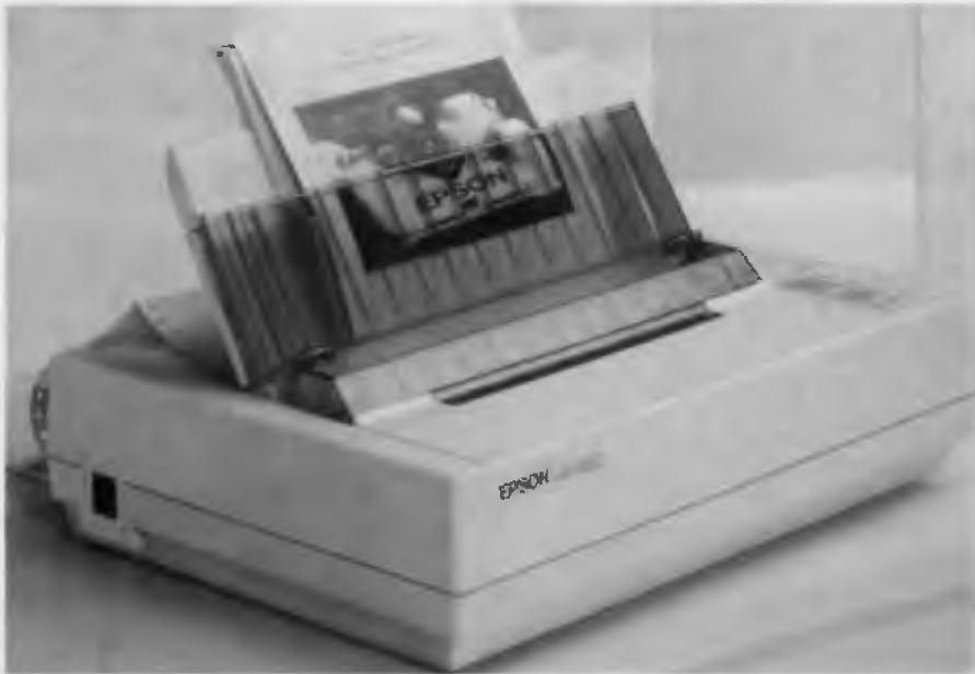
The Epson LQ-850 has a top-mounted lever to switch between tractor and friction feed (both standard).
