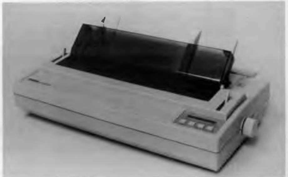
The 24-pin Epson LQ 2500+. The control panel allows access to many of the printer's settings, and can be used to set macros.
