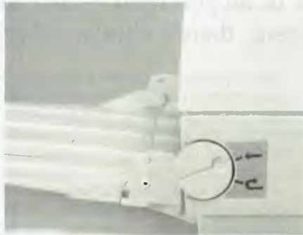
The Epson GQ-3500 has an 'exit selector' for face-up or -down output.
