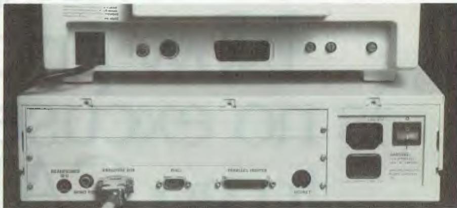
Figure 2. The rear panel of the system unit with a 32 ohm outlet for stereo headphones, a mono (composite) video adapter, the CGA adapter, the RS423 serial port, the Centronics parallel port, the Econet networking port and the power inlet and switch. At top left hand can be seen the two podule expansion units.
