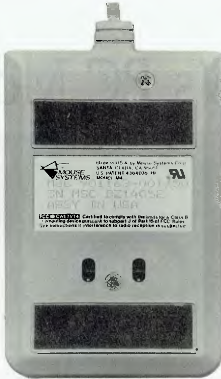
Figure 1. The PC Mouse has no moving parts — no wheels, balls or potentiometers. Instead, the mouse slides on felt pads over a reflective pad, which has a grid of vertical and horizontal lines printed on it. Movement of the mouse is sensed by reflection of the light from two LEDs, one of which emits visible red light and the other infrared light.
