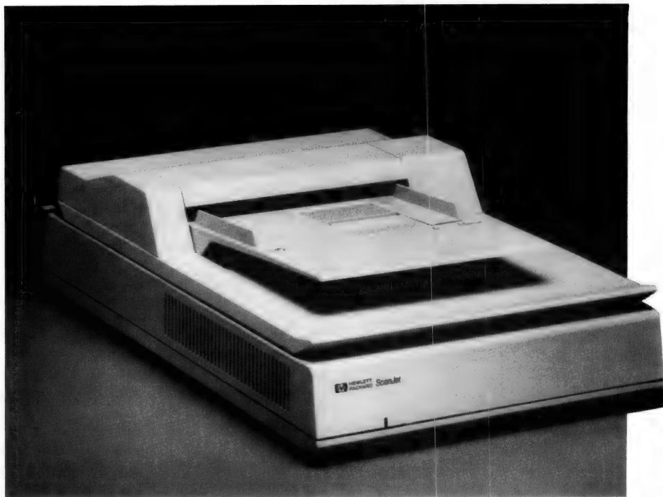
Figure 2. The Hewlett-Packard Scanlet is a good example of how far scanners have come in the past two years. For desktop publishing the scanner is best for optical character recognition — you do not, however, get a publishable result yet from scanning photographs.
