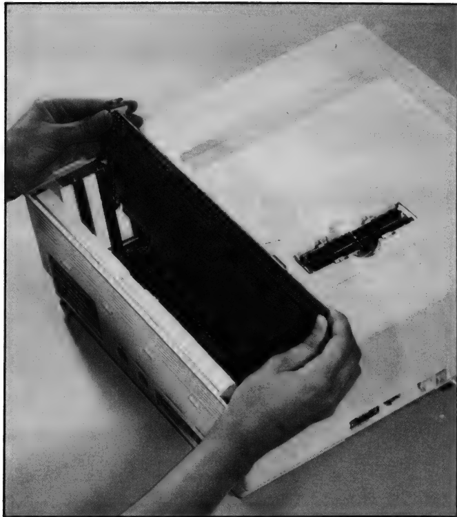
Lateral thinking! The PC1512s expansion slots run transversely which gives a much smaller footprint and allows easy access.
