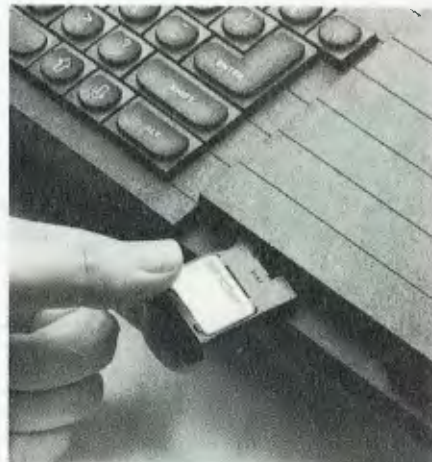
A tiny microdrive cartridge being inserted into the built-in microdrives.
