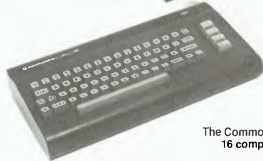
The new Commodore Plus/4 micro with four applications built into its ROM.
