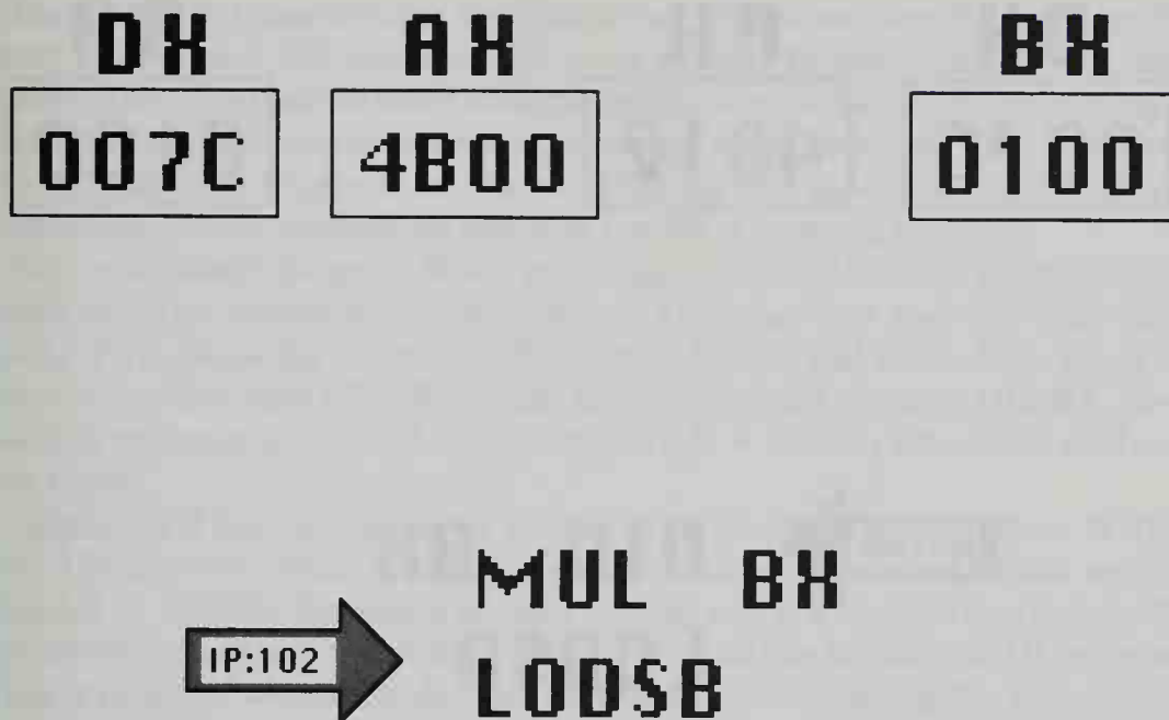
Figure 2-6. After we execute the MUL instruction: The result is in the DX:AX pair of registers.
